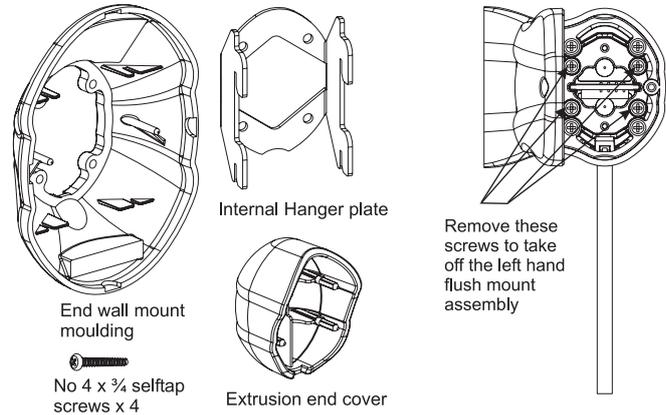
Fig 5-2: Kit Components Used for the Conversion
