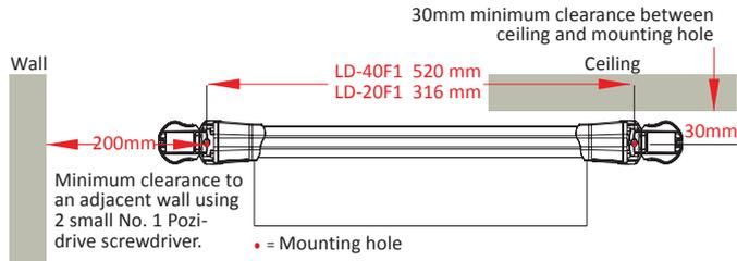
Fig 2-1: LD-20F1 & LD-40F1 Flush Sign Mounting Requirements
