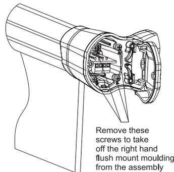
Fig 5-4: Removing the Right Hand Flush Wall Moulding
