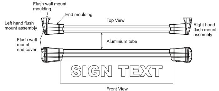
Fig 5-1: Sign Components to be Converted
