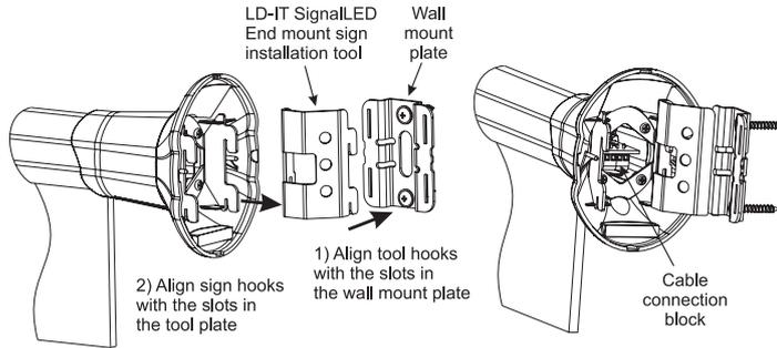
Fig 2-7: LD-IT End Mount Sign Installation Tool
