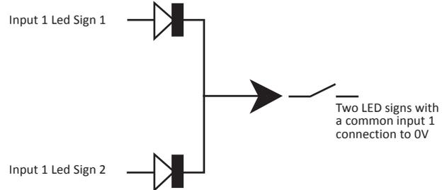
**Please note** pins 3 (0V) and 1 (input 1) are linked by default so that the sign will illuminate in its default mode when first powered up.
