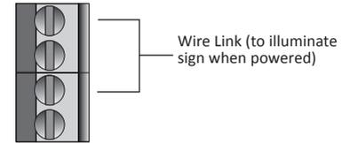
Fig 2-9: Wire link To Illuminate Sign When Powered
