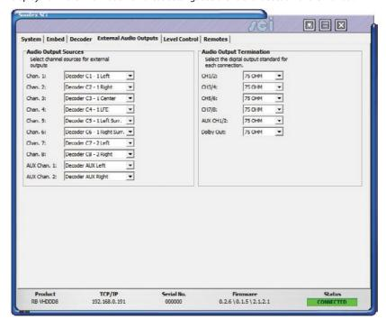
Fig 2-12: RB-VHDDD8 External Audio Screen.
