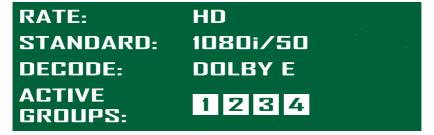
Fig 1-10: RB-VHDDD8 video input status screen.
