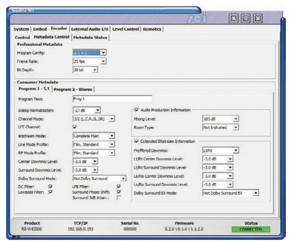
Fig 2-6: RB-VHEDD8 Encoder Meta Control Screen.
