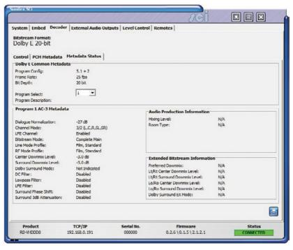
Fig 2-10: RB-VHDDD8 Decoder Metadata Status Screen.
