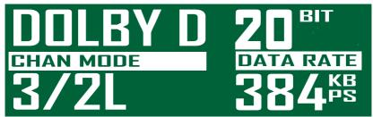
Fig 1-12: RB-DEDD8 Decoder Status Screen when decoding Dolby Digital.
