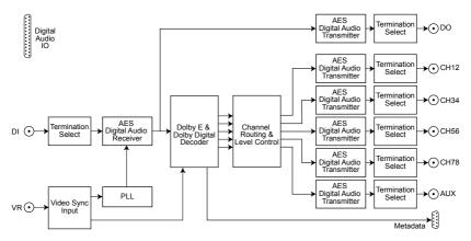
Fig 1-3: RB-DEDD8 System Block Diagram.
