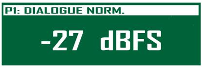
Fig 1-13: RB-DEDD8 Metadata Status Screen showing the Dialogue Normalization parameter.
