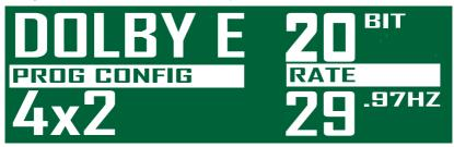
Fig 1-11 RB-DEDD8 Dolby Decoder Status Screen when decoding Dolby E.
