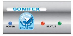
Fig 2-2: PS-SEND Power & Status LEDs
