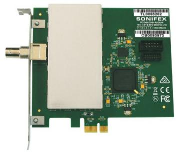
The PCIe DAB+/DAB radio capture card receives and decodes the entire contents of up to four DAB+/DAB ensembles, rendering each audio service as a virtual Windows audio capture device for use with multi-channel recording or monitoring software.
