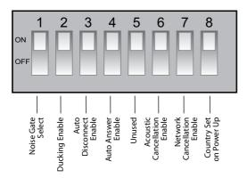
Figure 2-3: Configuration Settings Switches.
