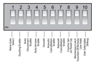
Figure 2-7: DHY-03EC Configuration Settings Switches.
