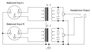
Fig 1-5: CM-HPX1 Block Diagram
