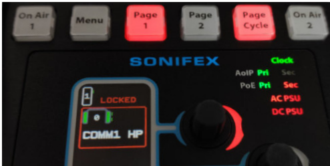
Fig 6-40: Locked user button warning
