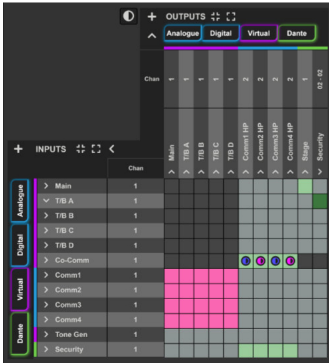
Fig 6-27: Routing talkback bus to a Dante output group
