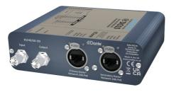
The easiest way to connect legacy SDI equipment to the Dante® network, the AVN-DIO10 can be used for simultaneous embedding and de-embedding. This simple plug and play audio/video interface provides a convenient and elegant method of connecting legacy 3G/HD/SD-SDI equipment to the Dante® AoIP audio network.
