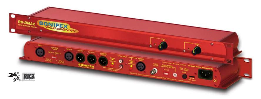
The microphone inputs are XLR-3 type and are electronically balanced. The input gain for each input can be adjusted individually by a volume control on the front panel enabling the use of dynamic and powered microphones and each has a LED level indicator. For each channel there are independent switches to control a high pass filter (low frequency roll-off at 125Hz) and to provide phantom power at +48V to the connected microphones.
