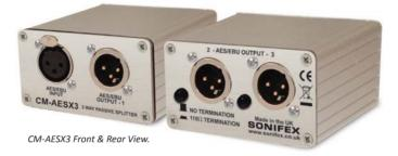
The CM-AESX3 is a passive "one-to-three" splitter housed in a small but robust aluminium box. It splits a single AES3 digital audio source to up to three destinations, using Neutrik XLR connectors.
