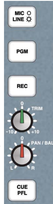
Fig 2-3: Mic/Line Channel Strip.
