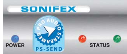
Fig 2-2: PS-SEND Power & Status LEDs
