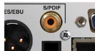
Fig 3-11: PS-PLAY S/PDIF Output
