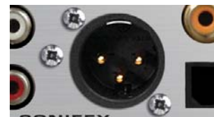
Fig 3-10: PS-PLAY AES/EBU Output
