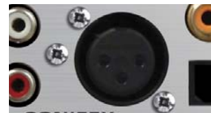
Fig 2-8 PS-SEND AES/EBU Input
