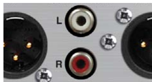
Fig 3-9: PS-PLAY RCA Phono Analogue Outputs
