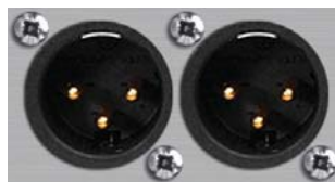
Fig 3-8: PS-PLAY Analogue Outputs
