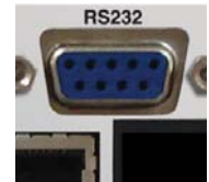
Fig 3-15: PS-PLAY RS-232 Serial Port
