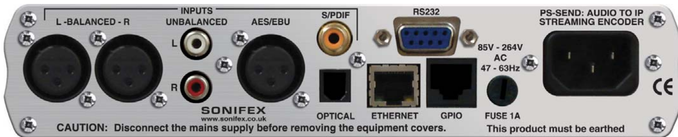
Fig 2-5: PS-SEND Rear Panel
